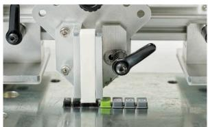
This test considers the wear that a calculator experiences from repeated use. A number of keys are examined, such as the number keys, the AC key, and function keys. The calculators are checked for wear by repeatedly moving them side to side while rubbing them through the use of an abrasive agent defined under Casio's internal standards.
