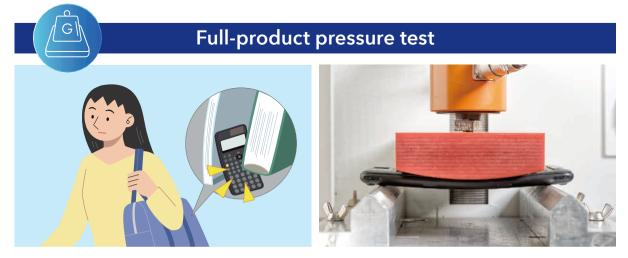
This test considers the kinds of stressors that might be placed on scientific calculators when they are pressed on by study materials or other external pressures, such as when the calculator is carried inside a bag on the way to school. In this test, both ends of the calculator are secured, and pressure is applied to the central portion of the device to test its durability.
