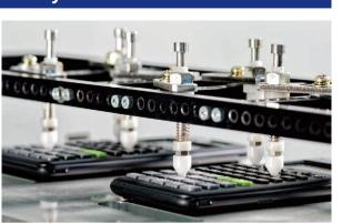
In this test, a machine is used to press the keys repeatedly to check the durability of the keys during repetitive operations.
